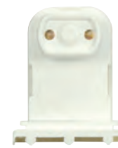
80-2312 Fixed Slide-On Shallow Base For T8 & T12 Lamps Accepts No. 18-16AWG Solid Wire Strip Wire 3/8" or 5/8" Quickwire Terminals 1 3/4" H x 1 1/2" W x 1 1/4" Dia. 660W-600V
