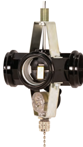
90-1588 4 Light Cluster Socket On-Off Nickel Pull Chain 1 3/4" 1/8 IP Threaded Top Bracket w/ 1/2" Nipple 1 3/4" 1/8 IP Threaded Bottom Bracket 7" AWM B/W Leads 105°C 660W-250V
