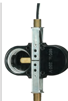
80-1664 Twin Offset 1 1/2" 1/8 IP Threaded Top Bracket w/ 3/8" Nipple 1 1/2" 1/8 IP Threaded Bottom Bracket w/3/8" Nipple 12" AWM B/W Leads 105°C 660W-250V
