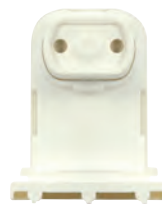
80-2311 Plunger Slide-On Shallow Base For T8 & T12 Lamps Accepts No. 18-16AWG Solid Wire Strip Wire 3/8" or 5/8" Quickwire Terminals 1 3/4" H x 1 1/2" W x 1 1/4" Dia. 660W-600V
