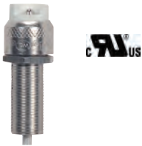
80-1914 6" SF-1 200°C Leads R7S Base, Halogen Socket w/1 1/8" Nipple 16 Ga. Wire 1 7/8" L 1000W-250V
