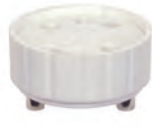
80-2511 White GU24 to GU24 Extender Overall Ext. 5/8" 660W-600V
