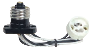
80-2368 Brown Medium Based Phenolic E26 Flanged Adapter to GU10 w/10" 18GA 105°C Leads, Overall Ext. 1/2" 660W-250V
