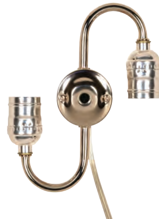
80-1272 Nickel Twin Keyless with 14" 18/2 SPT-2 105°C Clear Silver Wire Internal Wire - 18 AWM 105°C 7" Centers 1/8 IP Top and 1/8 IP Bottom 660W-250V
