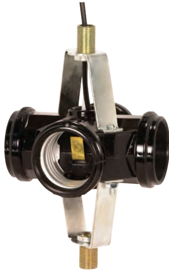
90-464 4 Light Cluster Socket 1 3/4" 1/8 IP Threaded Top Bracket w/ 1/2" Nipple 1 3/4" 1/8 IP Threaded Bottom Bracket w/ 1/2" Nipple 12" AWM B/W Leads 105°C 660W-250V
