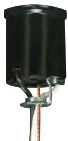
80-2036 Medium Base w/Rim 1/8 IP Hickey 12" AWM B/W 105°C Leads & Ground Wire Overall Ht. 2" Dia. 1 1/4" 660W-250V
