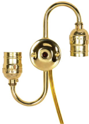
80-1189 Brite Gilt Twin Keyless with 14" 18/2 SPT-2 105°C Clear Gold Wire Internal Wire - 18 AWM 105°C 7" Centers 1/8 IP Top and 1/8 IP Bottom 660W-250V
