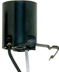
90-595 Snap-In Socket Bracket Extends 1/2" from End of Socket 7" AWM B/W Leads 105°C Ht. 1 1/2" Dia. 1 1/4" 660W-250V
