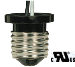
80-1970 Brown Medium Based Phenolic E26 Flanged Adapter w/10" 18GA 105°C Leads Overall Ext. 1/2" 660W-250V
