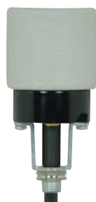
80-1755 Bottom Turn Knob Phenolic & Porcelain Shell Screw Terminals 1/8 IP Ht. 2 1/2" Dia. 1 1/2" 3/8" Bushing 660W-250V
