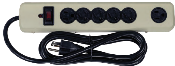
91-232 6' 14/3 SJT w/ Straight Plug 6 Outlet Metal Strip, Lighted On-Off w/Built-In Circuit Breaker, 300 Joules Rating, Surge Indicator Light, 1 Adapter Receptacle 15A-120V-1875W Packed 12
