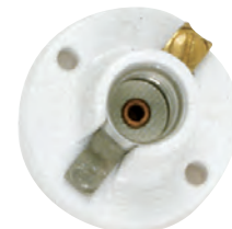
90-532 Candelabra Base Plastic Receptacle 7/8" H x 1 3/8" Dia. Screw Holes 1 1/8" CC 75W-125V
