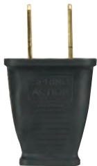
80-2408 Black Polarized Plug 2 Pole - 2 Wire 15A-125V
