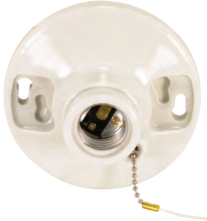
90-443 2 Terminal 90-2639 7" AWM B/W Leads 105°C Glazed Porcelain On-Off Pull Chain Ceiling Receptacle Screw Terminals 4 3/8" Dia. 250W-250V
