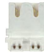
80-1937 Medium - Straight-In For 20GA Panel Slide-On - G13 Base Quick Connect No. 18GA Non-Shunted 1 3/8" H x 1 1/8" W x 3/4" Dia. 660W-600V
