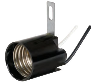
80-2163 Straight Bracket w/Hole Bracket Extends 1" from End of Socket 8" AWM B/W Leads 105°C CSSNP Ht. 1 1/2" Dia. 1 1/4" 660W-250V
