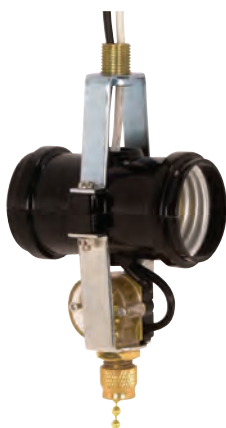
90-415 On-Off Brass Finish Pull Chain 1 1/2" 1/8 IP Threaded Top Bracket w/ 3/8" Nipple 1-3/4" 1/8 IP Threaded Bottom Bracket 12" AWM B/W Leads 105°C 660W-250V
